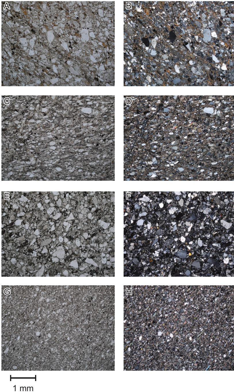
Fig. 5. Representative thin section photomicrographs from sampled units of four formations of the Fredericton Trough. PPL: plane polarized light, XPL: cross polarized light. (A) Digdeguash Formation, NA003A, PPL. (B) Digdeguash Formation, NA003A, XPL. (C) Flume Ridge Formation, NA010A, PPL. (D) Flume Ridge Formation, NA010A, XPL. (E) Hayes Brook Formation, NA005A, PPL. (F) Hayes Brook Formation, NA005A, XPL. (G) Burtt's Corner Formation, NA001A, PPL. (H) Burtt's Corner Formation, NA001A, XPL.
