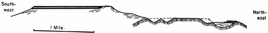
Fig. 2. Diagrammatic structural cross-section of Isspah Butte and area to the northeast, showing flat-lying lavas (wide horizontal lines), the underlying breccias (dash-dot lines inclined parallel to the stratification) resting on an erosion surface developed on folded Permian sediments (steeply inclined line pattern). Pre-volcanic surface indicated by dashed line. Two buried valleys and three recent valleys have been cut below the level of the peneplain surface. The breccias in the middle and northeastern part of the section strike parallel to the line of the section and dip at angles of from 10 to 25 degrees.
