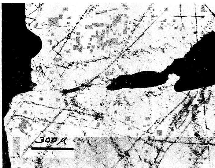
B. Near fault zone, partially healed fractures decorated with inclusions ("type 1" fractures of text) are abundant, they are also present within blocks and breccia clasts of the fault zone itself.
