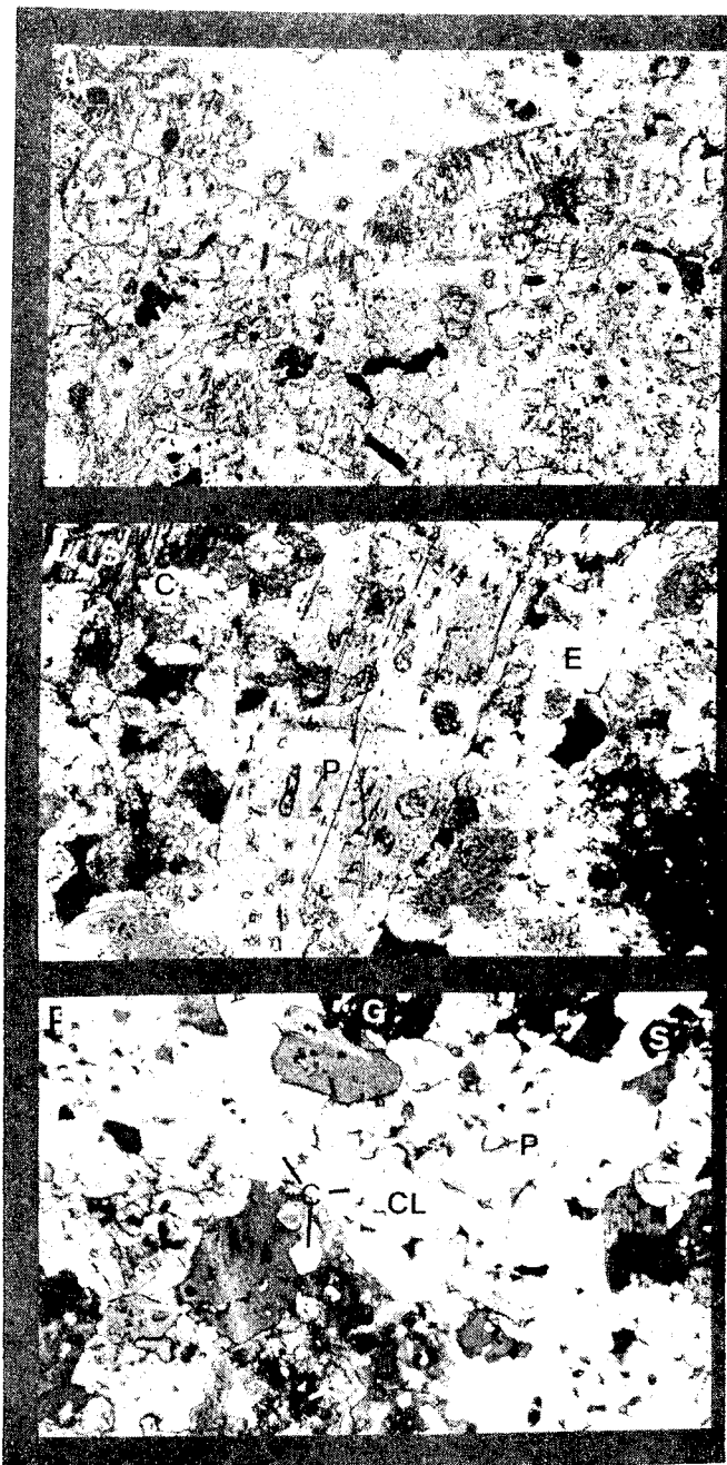
A. Photomicrograph showing magnetite (M) inclusions in pyroxene (P) and garnet (G). Stage I, Massive skarn. Plane light. \times 6.3 .
