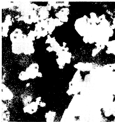
C. Grain boundaries disappear near the concretion margin and only rarely can framboidal remnants be detected in the euhedral aggregates. Picture width 180 \mu\text{m} , oil immersion.
