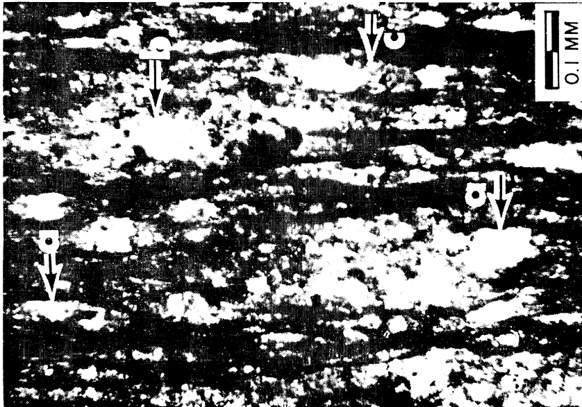
A. Photomicrograph of (a) grains truncated on one side, (b) normal (equant) grains, and (c) pressure shadows. B. Photomicrograph of (a) grains truncated on two sides, (b) normal (equant) grains, and (c) pressure shadows.
