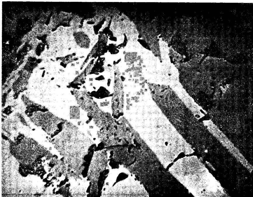
G. Euhedral diopside crystals (darker) in andradite. JCA 01, 1000 \times .
