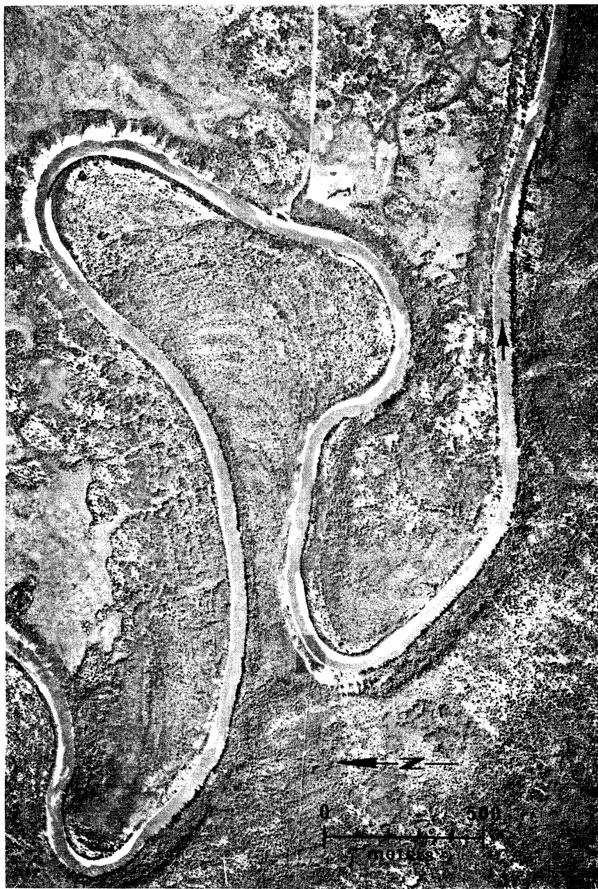
A "T" meander pattern produced by the formation of upstream and downstream channel lobes on a simple type A bend. Channel migration has destroyed much of the original point-bar surface; note the truncated scroll-bars. British Columbia air photo BC7185-065.
