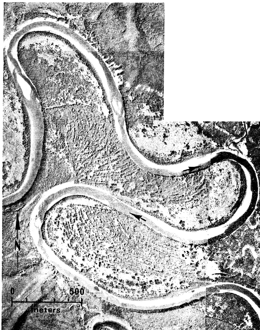
A typical "T" meander pattern on the Beatton River. Note the development of the "goose-neck" and the various phases of lateral migration indicated by the vegetation pattern. British Columbia Government air photo BC7303-052.
