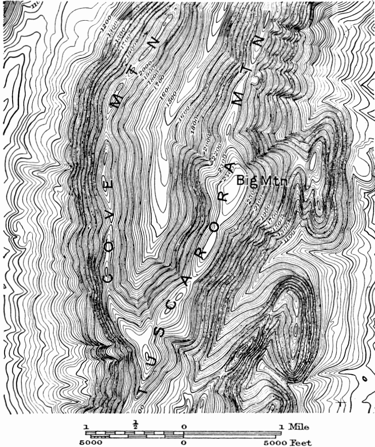
Fig. 3. Contour map of Big Mountain, Tuscarora Mountain, and Cove Mountain, east of McConnellsburg, Pennsylvania, showing parts of Schooley peneplain over 2400 feet altitude.
