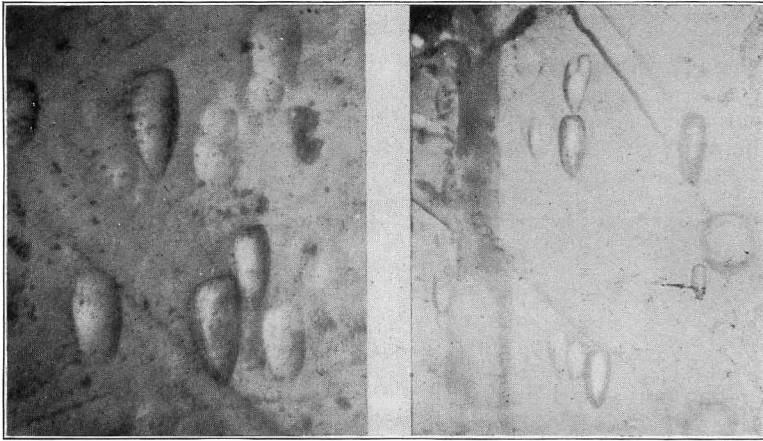
FIGS. 2, 3. Kaersutite from Linosa . Etch pits on 110, HF. Fig. 2, \times 360 ; fig. 3, \times 240 .
