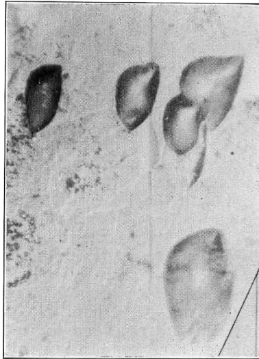
FIG. 7, Kaersutite, Kaersut, Greenland. Etch pits on 110, HF; \times 480
