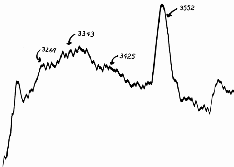
Fig. 1. Microphotometer tracing of the spectrum of O-H bands in \text{Na}_2\text{B}_4\text{O}_7 \cdot 4\text{H}_2\text{O} .
