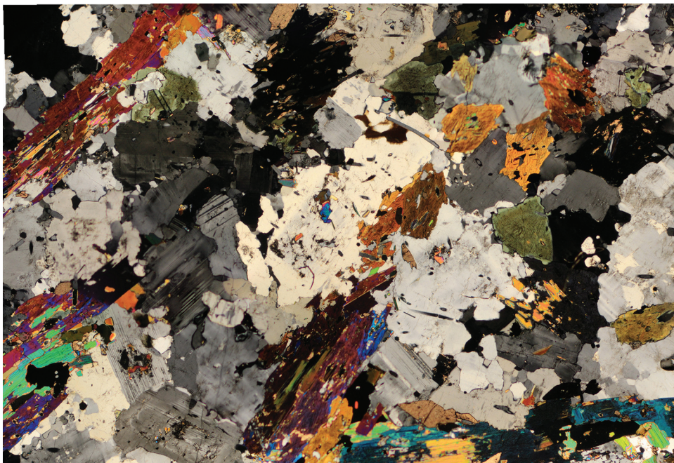
Fig. 2. Photomicrograph of the Wamsutta Diorite showing elongated amphibole grains, plagioclase, and titanite. Field of view is 10 mm.
