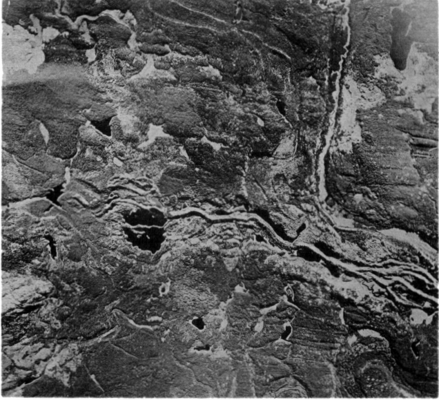
Fig. 1. MACKINNON COMPOUND ESKER EAST OF SALMON RIVER. The single ridge in the centre of the photograph occupies a trough-like valley 150 feet deep.
