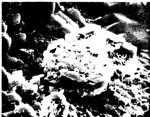
Euhedral and twinned authigenic K-feldspar crystals on the etched surface of basaltic glass, at the basalt/sediment interface, DSDP Site 322, Bellingshausen Abyssal Plain. White line represents 30\mu\text{m} .
