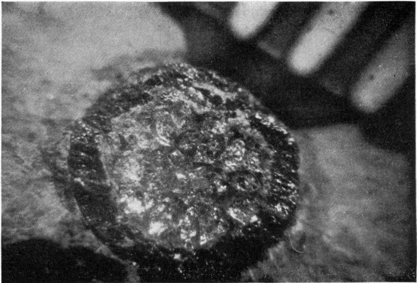
Fig. 3. Synthetic garnet, \times 24 .
