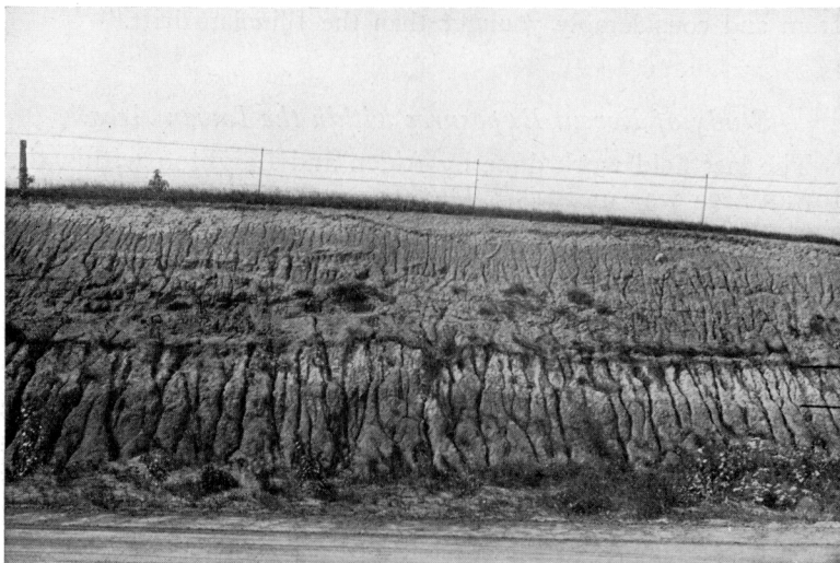
Fig. 1. Road cut near the middle of the north line of the northeast \frac{1}{4} , Section 16, Windsor township, Fayette county, showing Kansan gumbotil overlain by Loveland loess, overlain by Iowan till, overlain by Peorian loess.
