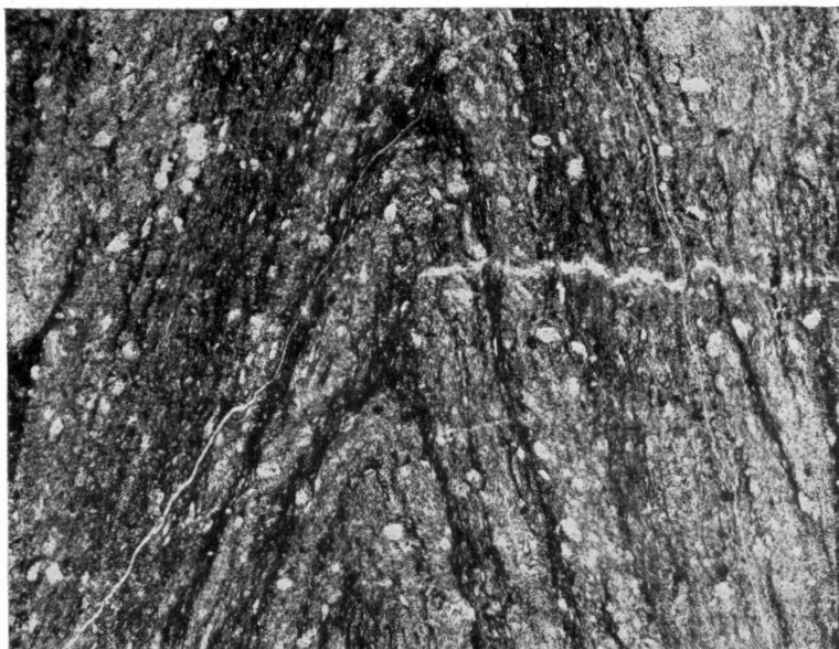
Fig. 8. Photomicrograph showing folded flow bands in ultramylonite. Note the secondary quartz veinlets cutting the flow structure. Crystal Springs Lakes, California (Nicols uncrossed, x 60).
