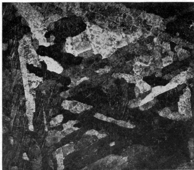
Fig. 3. The Widmanstätten Pattern of the Cañon Diablo Meteorite. x 1.5. Streaks which appear to be scratches are Neumann Bands.
